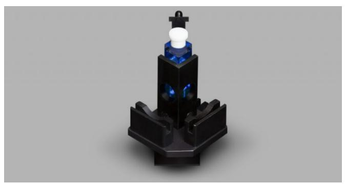
Single cuvette holder, temperature adjustable by water/coolant circulation, fitted with integrated probe for sample temperature monitoring by spectrometer operating software. Filter slots are provided for holding 50 mm square filters. This sample holder is included as part of the standard system.
