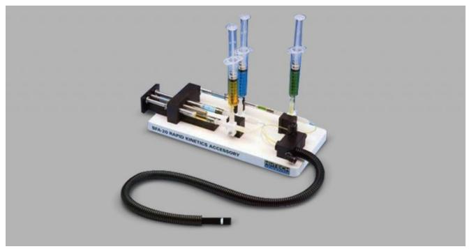
Rapid kinetic accessory for multi-mixing capabilities. Comprises sample handling unit, fitted with three 1 ml drive syringes, 600 mm long umbilical, pneumatic drive system and square mixing/observation cuvette with standard dimensions (10 mm). Includes slotted sample chamber lid to allow the cuvette to be fitted to the FLS980. Manual control.
