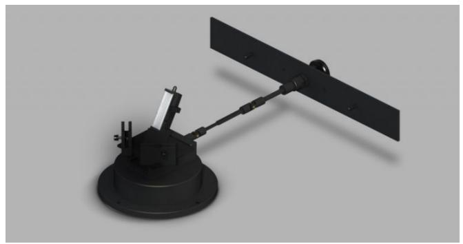
The front face sample holder has external adjustment for accurate sample positioning. The accessory comes with inserts for demountable cuvette film/slide clamp and holder for microsamples.
