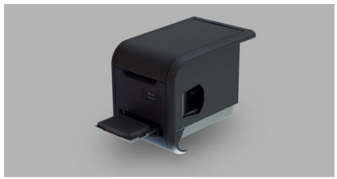
The Multiwell-plate reader is an external module that is attached to the FS980 to perform spectral or time resolved measurements on multi-well plates. The multiwell plate reader module is coupled to the FLS980 by means of a bifurcated optical fibre. The control of the module is fully automated from the F980 software, temperature near the well plate is recorded. Spectral range depends on FLS980 spectrometer configuration and bifurcated fibre assembly. 96 well and 384 wells are available.
