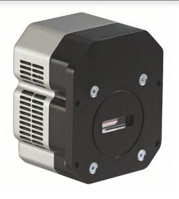
A choice of CCD, EMCCD and InGaAs detectors are available with a maximum of 4 detectors being integrated per system. For fluorescence lifetime measurements, single photon counting detectors can also be integrated.
